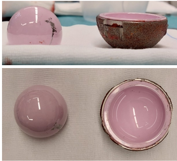
Fig. 4 — Cup and head after removal, showing no macroscopic signs of wear.
