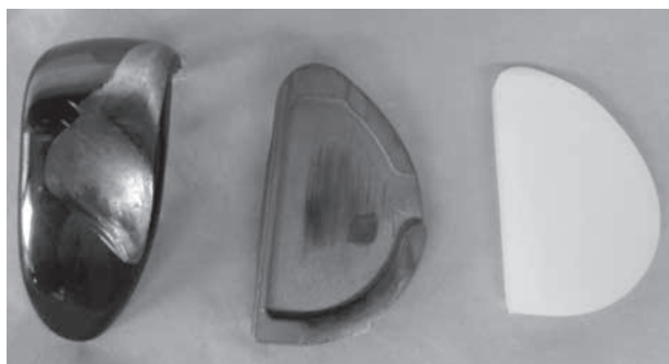
Fig. 4. — Components explanted which presented a major defect of the posterior part of the femoral implant, a minor defect of the tibial component and an intact PE.
