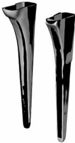
Fig. 5. — Overlay of rasp (grey) and stem (black) geometry, for CBC-T (left) and CLS stem (right). Note that the mid-shaft area of the CLS stem shows stem oversize because of the absence of teeth on the rasp (see also Figure 2).
