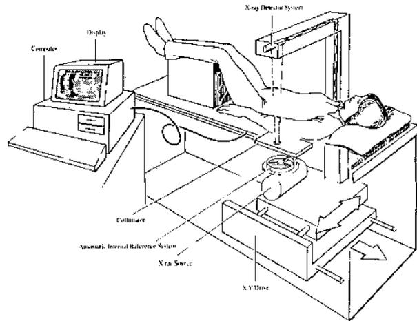
Fig. 1. — Components of the Hologic QDR-1000 x ray bone densitometer — measurement technique (see text).
