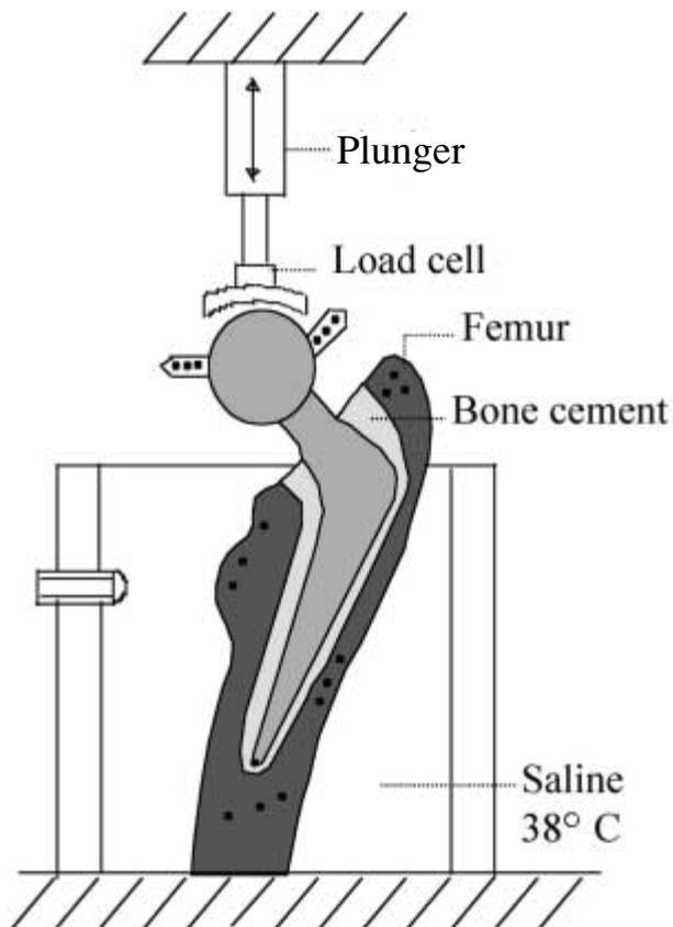
**Fig. 1.** — Schematic representation of the experimental set-up showing the fixated reconstruction and the loading plunger of the MTS machine. RSA markers were attached to the prosthesis (six to the prosthetic head and one to the tip of the prosthesis) and the bone. Testing environment was saline at 38°C.
