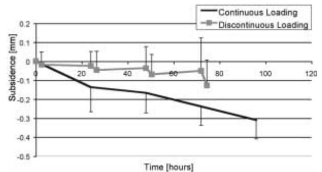
**Fig. 2.** — Average subsidence curves as a function of time (hours). The continuously loaded specimens show a continuous subsidence patterns. The discontinuously loaded specimens subside only during the relatively short loading periods and seem to recoil a little during the unloaded periods. Error bars indicate the standard deviations of the 5 measurements.
