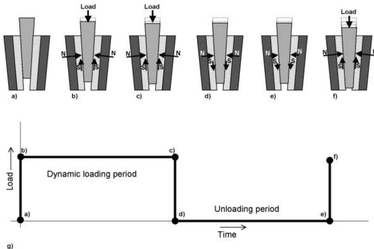
**Fig. 4.** — Schematic representation of the subsidence and interface stresses in a tapered stem surrounded by a cement mantle and bone. These quantities are shown before and after a loading period and after an unloading period.
