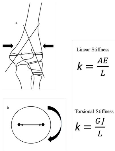
**Figure 4.** — Rigidity of pinning fixation against different force at fracture site. a) Translational force; b) Torsional force; Arrow = direction of force; Line = length of working distance;  $k$  = stiffness,  $E$  = elastic modulus,  $A$  = cross-sectional area;  $L$  = length of working distance;  $G$  = rigidity constant,  $J$  = torsion constant.
