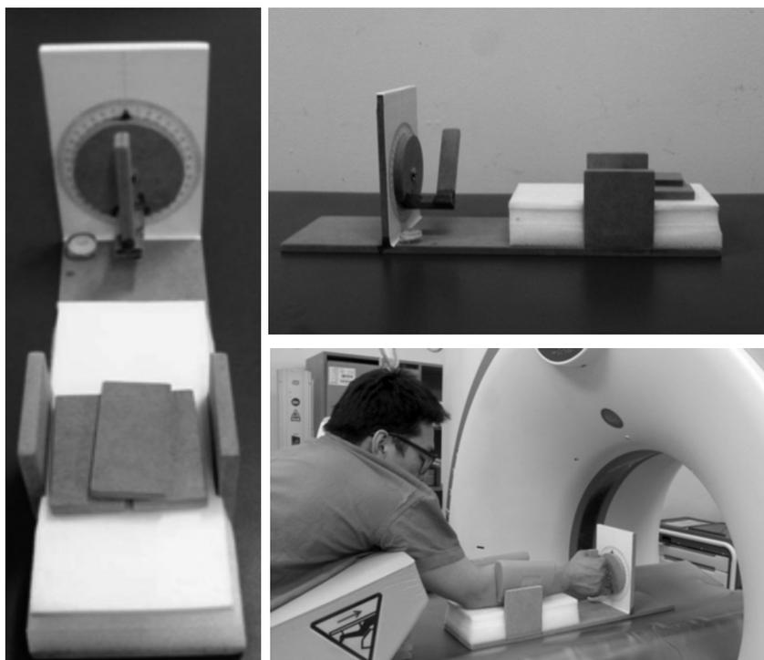
**Figure 4.** — In order to measure the range of motion of the forearm, we produced our own version. The middle scale can be measured from neutral, 0 degrees to pronation 90 degrees and supination 90 degrees, with a minimum unit of 1 degree.
