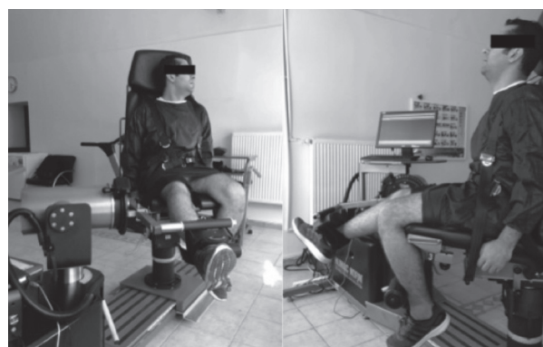
Fig. 1. — A demonstrative view of proprioception measurements, which were done by the isokinetic dynamometer (HUMAC® NORMTM Testing & Rehabilitation System, USA). Active and passive sensation of the patients at 30° and 60° were evaluated.
