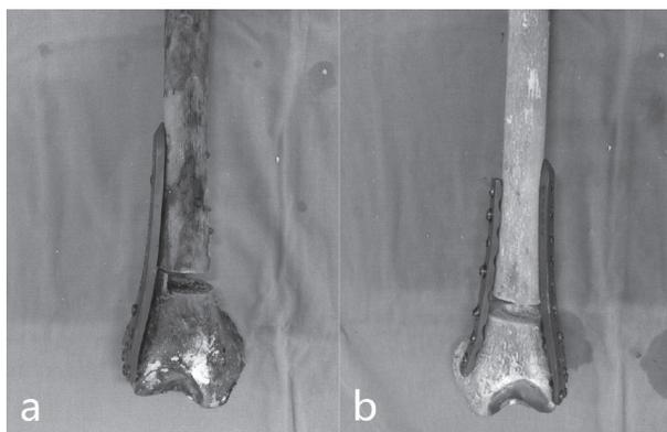
**Fig.1.** — Paired instrumented femurs prepared with a transverse 1-cm osteotomy gap to simulate a metaphyseal fracture with comminution. a. single lateral plate; b. double plating
