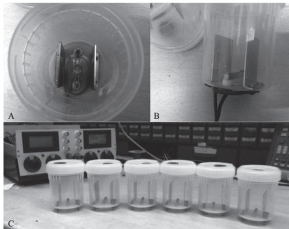
**Fig. 1.** — Photography of the used recipients showing the different metallic and electric components of the bottles. A) Top view of the recipient, showing the circular plates introduced in the bottle and flanked by two rectangular plates. B) Lateral view of the recipient, the electric connections can be seen below. C) General view of the recipients containing the plates.
