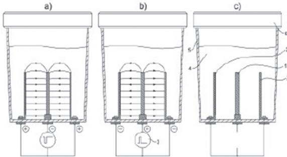
**Fig. 2.** — Drawing of the electric field distribution of the three different electric models: a) Plate negatively charged, b) Plate positively charged, c) Control plate without current). Detail of numbers: 1- Plate Under Test or circular metal plate; 2- Lateral L-plates; 3- pulse wave generator; 4- liquid medium with bacteria; 5- container for urine sample; 6- tight cover that keeps sealed the recipient.
