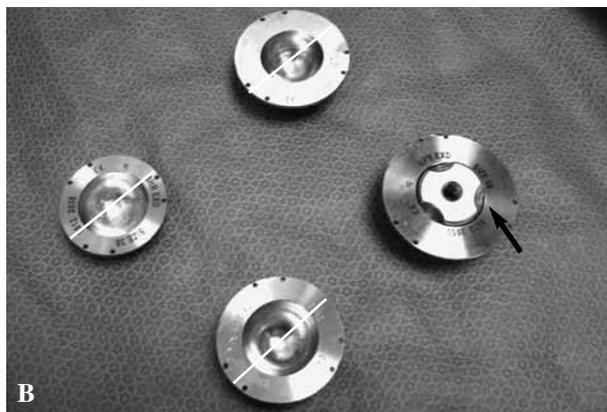
**Fig. 2B.** — The ‘adaptor surface’ of the Explant™ adaptor device. This picture shows variations in the diameter (white lines) to accommodate various cup sizes with the standard 28 mm recess for the centering head of the Explant™ (arrow).
