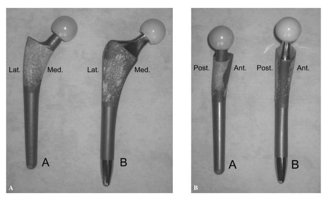
*Fig. 1.* — Profile<sup>®</sup> (DePuy Orthopaedics, Warsaw, USA) (A) and Image<sup>®</sup> (Smith & Nephew, Memphis, USA) (B) uncemented stem. Ant. = Anterior, Post. = Posterior, Lat. = Lateral, Med. = Medial. Both implants were retrieved during revision surgery and have different sizes.
