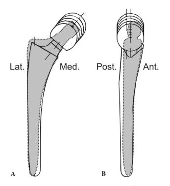
*Fig. 3.* — Superposition of the templates of a Profile<sup>®</sup> stem size 11 (white, —) and an Image<sup>®</sup> stem size 2 (gray, …). Both stems have similar dimensions. In the AP view (A), the Image<sup>®</sup> stem is bulkier in the proximal 1/3, but not in the lateral view (B). In both views, the Image<sup>®</sup> stem is thinner distally. Ant. = Anterior, Post. = Posterior, Lat. = Lateral, Med. = Medial.
