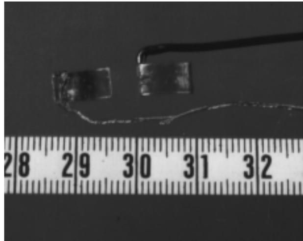
Fig. 1. — Implantable force transducer (IFT)
