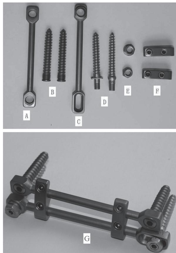
**Fig. 1.** — The components of the D-rod system. (A) Locking rod. (B) Locking screw (6mm in diameter). (C) Distraction/compression rod (60 to 130mm). (D) Bolts. (E) Nuts. (F) Adjustable transverse link bar. (G) Overall relation of the D-rod system.
