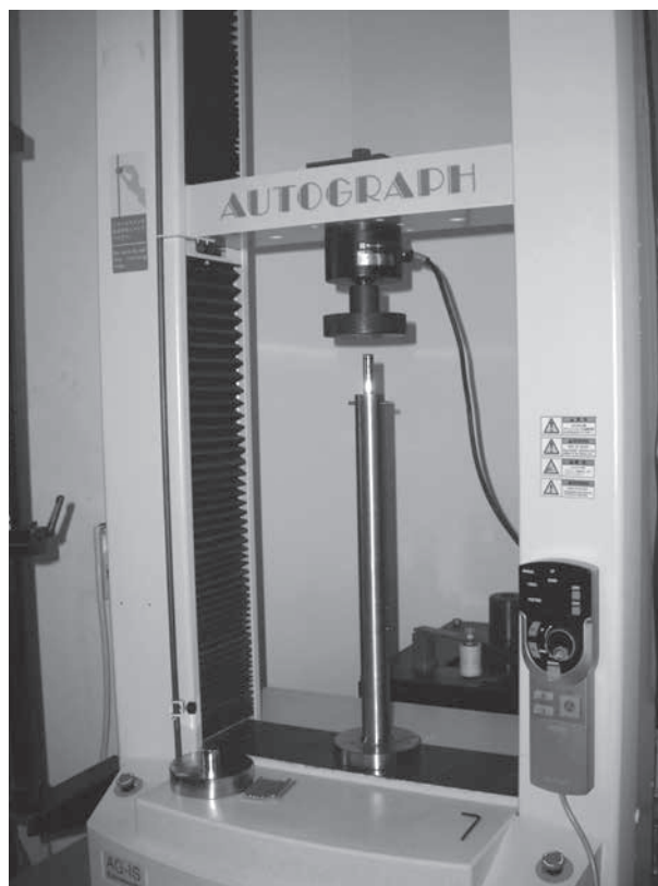
Fig. 3. — Three-point bending test of the nail with compression tube using an axial compression testing machine.
