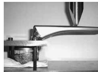
**Fig. 3.** — Lever-out test simulated femoral neck impingement with the liner lip acting as the fulcrum.
