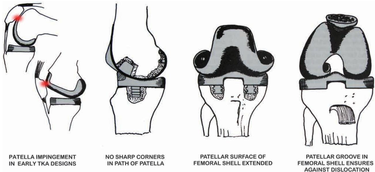
**Fig. 9.** — Failure to accommodate the patella in early arthroplasty designs resulted in patello-femoral impingement (areas denoted in red) and anterior knee pain. The 3 images on the right denote design alterations suggested by Seedhom in 1974 to overcome problems of impingement and to improve patello-femoral kinematics and function (91).
