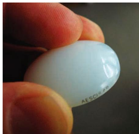
**Fig. 6.** — Focal area of polyethylene deformation (cold-flow) at the periphery of a retrieved patellar component, created through bifurcation of contact at flexion >70°. Changes considered to accommodate non-conformity between patellar implant and femoral condyle by creeping in ways to reduce contact stress. Component courtesy of Prof. W. Plitz, Ludwig-Maximilian-University, Munich.
