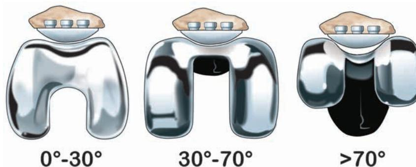
**Fig. 3.** — Contact position between patellar implant and femoral component at various degrees of knee flexion. Point contact in extension and early flexion, due to limited conformity between patellar implant and femoral flange ; line contact in mid-flexion ( $30^\circ$ - $70^\circ$ ), due to increasing conformity between patellar implant and trochlea ; bifurcation of contact area beyond  $70^\circ$  (Copyrights of illustration remain with author).
