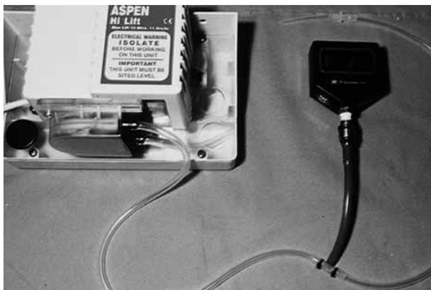
Fig. 2. — Pressure measurement apparatus.
