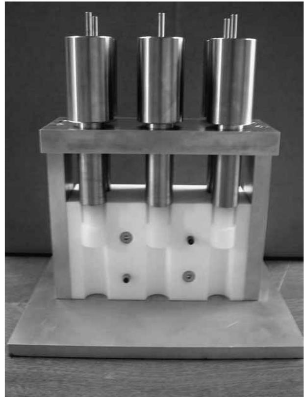
Fig. 2. — Experimental apparatus modified for multiple specimen processing
