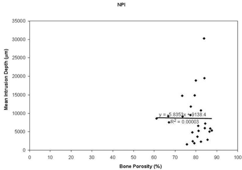
**Fig. 7.** — Scatter plot of porosity Vs mean intrusion depth for the negative pressure intrusion group showing no correlation between porosity and cement intrusion depth.
