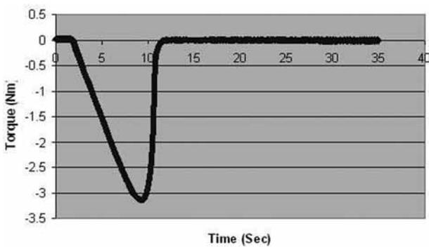
Fig. 5. — Graph of typical torsion test to failure
