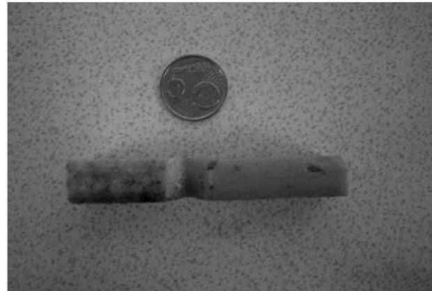
Fig. 3. — Machined cement bone construct
