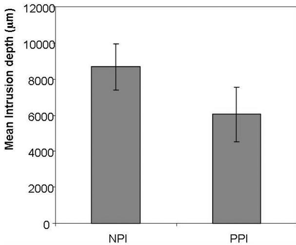
Fig. 4. — Mean intrusion depth for the negative pressure intrusion and control groups (error bars indicate 95% confidence intervals). Higher mean intrusion depth and lower variability was observed for the negative pressure intrusion group than for the control group.
