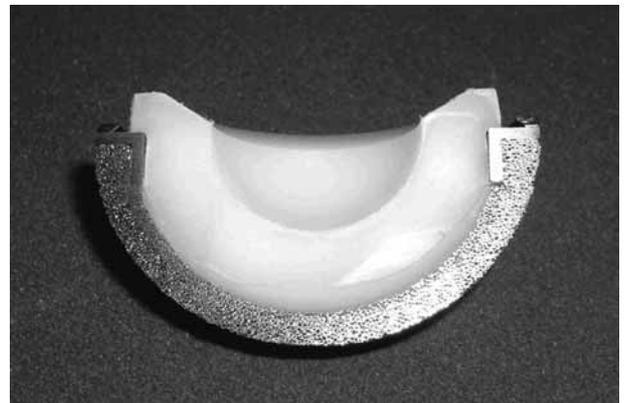
*Fig. 3.* — Hydrocel acetabular implant in cross-section, showing the bonding between the polyethylene and the tantalum shell.
