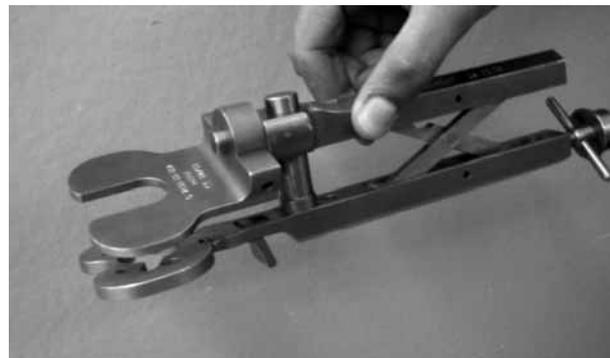
**Fig. 1.** — Spreader tool prototype – the lower plate rests on the tibial cut, the upper plate swivels and lifts the femoral condyles, as the soft tissues are put under tension by turning the screw.
