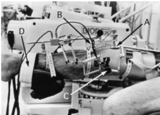
**Fig 1.** — The electrogoniometer system (CA-4000) fitted to a lower limb of a patient sitting on a Biodex seat. The removal arm is padded on the patella (A) and the tibial tuberosity (B). Potentiometer C is used to measure the knee joint angle and is aligned with the knee joint center. The resistance pad (D) of the Biodex is placed on the tibia just above the ankle joint.
