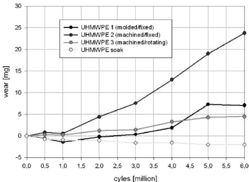
Fig. 2. — Wear vs number of cycles
