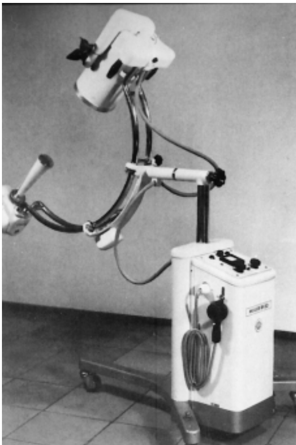
Fig. 9. — Probably the first image intensifier (BV 20) for surgical fluoroscopy designed by C. H. F. Müller in 1956.
